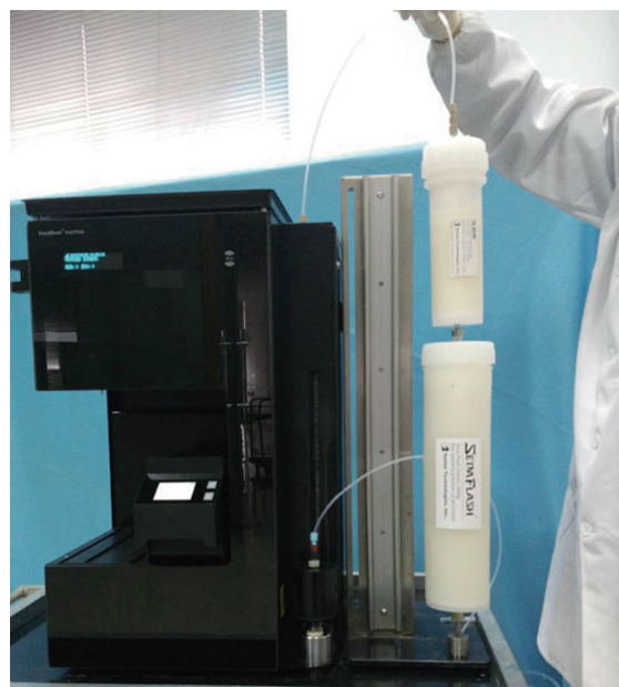
Figure 3. The experimental setup for automatic flash chromatography.
