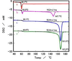
Figure 1 DSC results for cooling at 0.1°C/min
