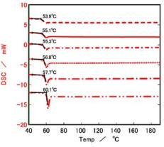
Quench cooling Cooling at 10°C/min Cooling at 5°/min Cooling at 1°C/min Cooling at 0.5°/min Cooling at 0.1°/min
