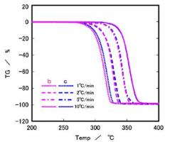
Figure 7 STA results for samples b and c for the following heating rates: 1°C/min 2°C/min 5°C/min 10°C/min
