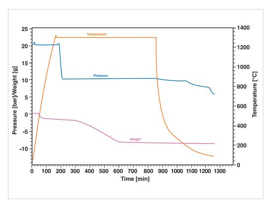
Example of coal sample being gasified under  $CO_2$  atmosphere
