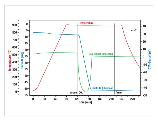
This application shows a typical measurement of a Charcoal gasification under Carbon Dioxide atmosphere at a pressure of 20 bar.
