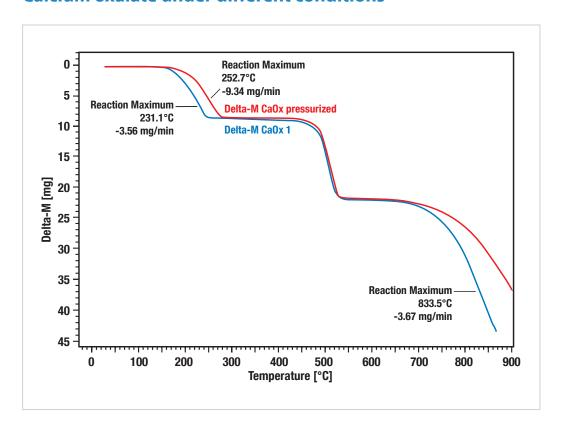
Comparison of Calcium Oxalate decomposition under Pressure (20 bar, red curve) vs. atmospheric condition (blue curve). A significant pressure dependence of the decomposition steps 1 and
