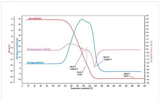
The dehydrate is raw gypsum. There are two molecules of water attached to a single CaSO<sub>4</sub> molecule. By heating up to app. 160°C the semi hydrate gypsum is built. 1,5 molecules of water are released; so two CaSO<sub>4</sub> molecules are sharing a single water molecule. By heating to higher temperatures (400°C) the anhydrate is built. This is the socalled "dead burned gypsum", also known as alabaster. In this state no water at all is attached to the CaSO<sub>4</sub> molecules.
