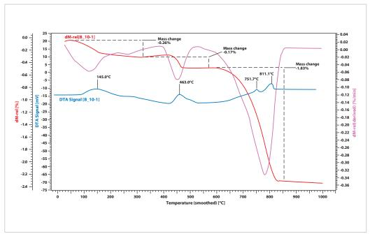
The main parts of cement are tri calcium silicate, di calcium silicate and tri calcium aluminates. Hydrates slowly form after mixing cement with water. The absorbed water evaporates first. Hydrates of the calcium silicate decompose at  $570^{\circ}$ C. The hydroxides of calcium, magnesium and aluminum follow. Subsequently,  $CO_2$  splits off from calcium carbonate.
