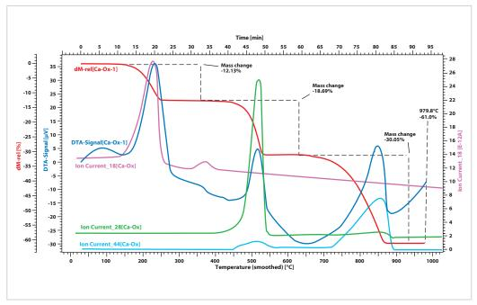
The evolved gases from the decomposition of calcium oxalate has been fed into the mass spectrometer with a heated capillary. The ion currents for mass numbers 18 (water), 28 (carbon monoxide) and 44 (carbon dioxide) have been imported into the graph.
