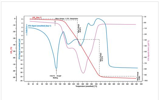
At the beginning of the heating process some adsorbed water is released, resulting in a weight loss of around 1%. At 140°C the melting point of the Aspirin is reached, resulting in an exothermic reaction, measured on the DTA trace. At 160°C the decomposition of the melted drug takes place in several stages. Since the decomposition products are volatile a weight loss of just about 80% occurs.
