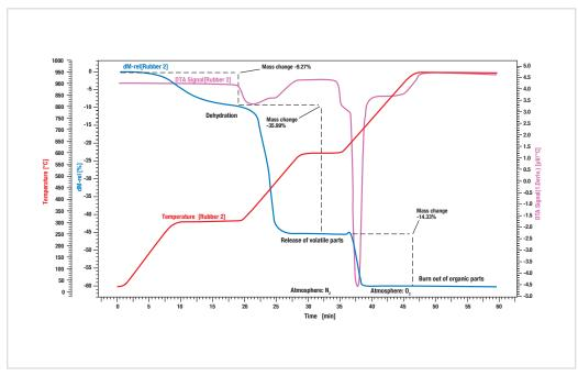
In the first step of weight loss, the dehydration of the sample takes place. The amount of water was 9.27%. In the second reaction step, the volatile components are released by pyrolysis under N<sub>2</sub> atmosphere. The amount of these components is 35.99%. For the third reaction step, the atmosphere is changed to O<sub>2</sub> - all organic components are burned out. The loss in weight is 14.33%. The remaining rest of 40.41% are inorganic components like ashes, slake or fillers.
