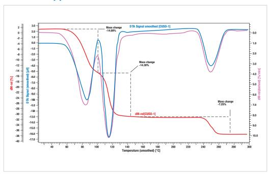
Inorganic salts first set their crystal water free. Vitriol of Copper heated with  $10^{\circ}$ C/min. results in a first TG stage, which corresponds to  $4H_2O$ . TG and DTA show that the curve is made up of two separate steps, one closely behind the other. At around  $250^{\circ}$ C the most strongly bound water evaporates.
