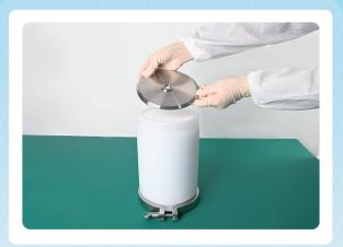
**Step 10** Place the other cap on the sealing ring, and the sealing ring fits into the groove on the lower part of the cap.
