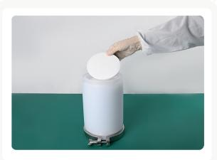
**Step 8** Place the top frit on the filled media bed and align the frit horizontally.
