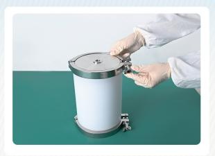
**Step 11** Use the other hoop to hold the outer rim of the cap and the outer rim of the column body opening, and lock the column body and the cap by screwing the locking nut. It is recommended to use a wrench tool to tighten the locking nut.
