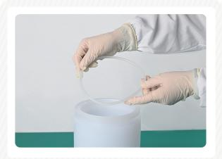
**Step 2** Place the column tube on the lab bench, and place the sealing ring in the groove of the column tube opening.
