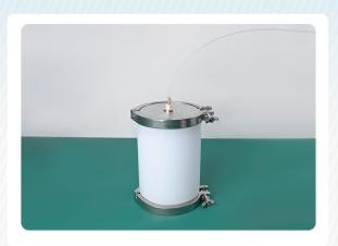
**Step 12** Connect the adaptors of the tubings to the inlet and outlet of the cartridge. Users can choose the appropriate adaptor of 1/8-inch, 3/16-inch or 1/4-inch OD tubing according to their needs.
