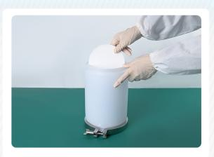
**Step 6** Rotate the column body so that the other opening end is up. Place the bottom frit into the lower part of the column body, and use the plug tool to flatten the bottom frit. At this time, the bottom frit is in contact with the cap.
