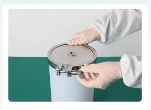
Step 5 The locking component on the hoop includes a screw rod and a locking nut, and the locking nut is threaded on the screw rod. Pass the screw rod through the locking opening, and screw the locking nut to make the column tube and the cap move toward each other to realize the locking connection. It is recommended to use a wrench tool to tighten the locking nut.
