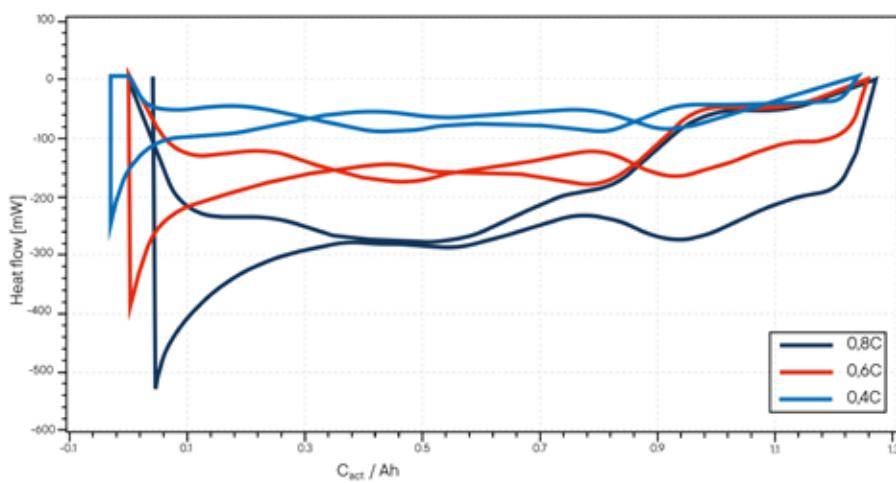
Heat flow over the capacity of a 1-cell Li-ion standard battery at different charge and discharge currents. This allows differences in the efficiency of various charging parameters to be displayed depending on the capacity of a battery. What is striking here, for example, is the different residual capacity depending on the different discharge parameters. A significant increase in heat flow at higher charging and discharging currents is also evident.
