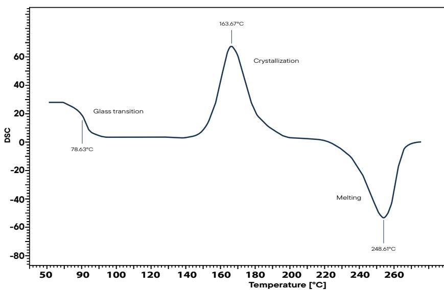
Depending on the cooling rate, the degree of crystallinity of the polymer changes significantly. During a subsequent heating run, cold crystallization can only be observed with a linear heating rate of 20 K/min. The curve reveals a distinct glass transition around 80 °C, followed by cold crystallization of the amorphous regions starting at approximately 148 °C and a melting peak at 230 °C. This allows for complete characterization of the sample with just two heating cycles.
