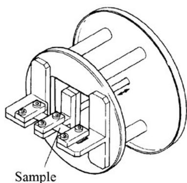
**Figure 1** Film shear measurement head used in DMA7100
