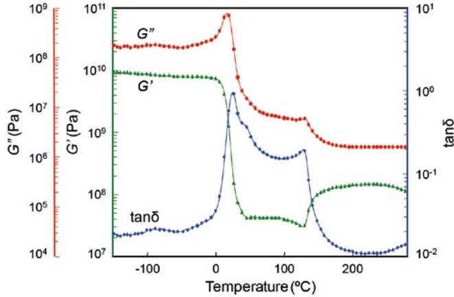
**Figure 2** Viscoelastic spectrum of Carbon fiber reinforced epoxy prepreg (1st heating) Frequency: 1Hz
