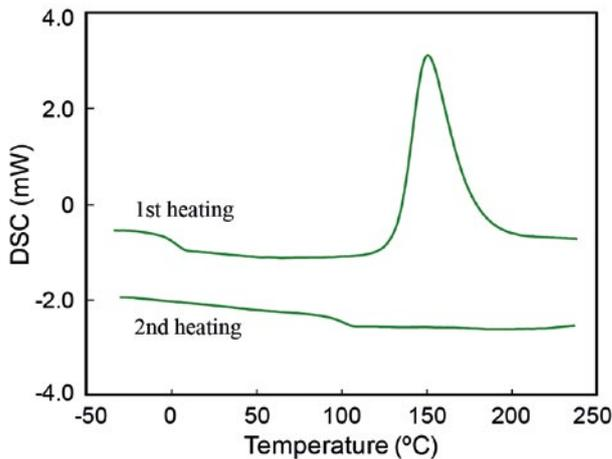
**Figure 4** DSC curves of Carbon fiber reinforced epoxy prepreg Heating rate: 10°C/min
