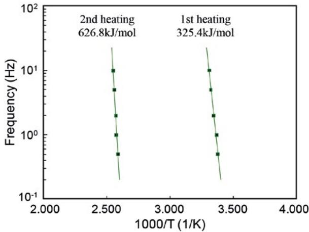
**Figure 4** Apparent activation energy of primary dispersion of 1st and 2nd heating
