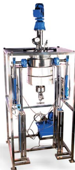
50 ltr with hydraulic vessel raising lowering
