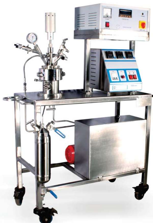
500 ml high pressure vessel with ultrasonicator probe system
