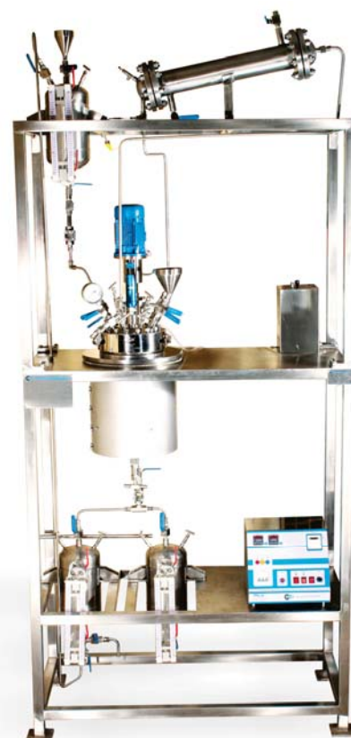
5 ltr reactor with charging & condensation arrangement
