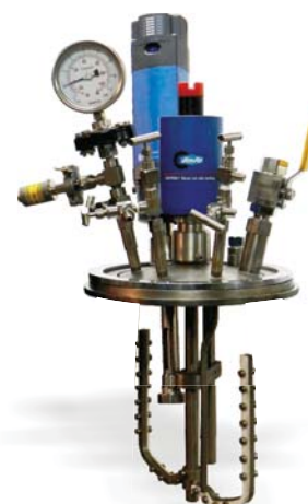
25 ltr titanium high vacuum reactor lid with homogenizer & anchor with PTFE wiper blades
