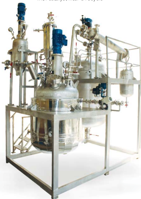
500 Ltr hydrogenation pilot plant with catalyst filter & recycle
