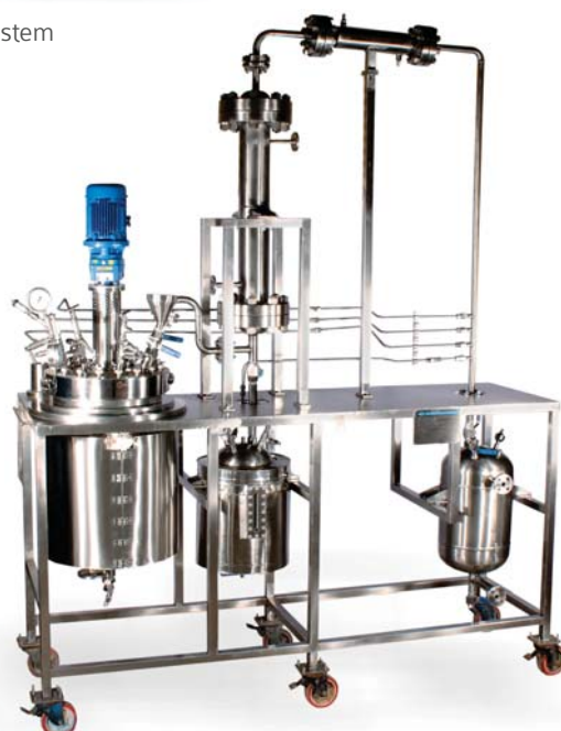
100 ltr pilot plant with distillation setup
