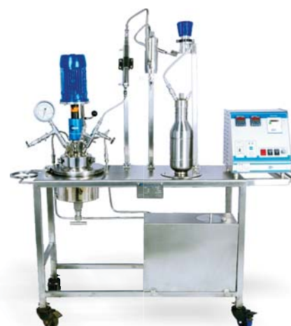
Batch reactor for visbreaking process
