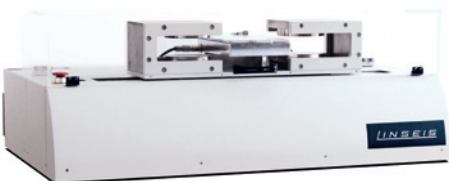
TFA with permanent magnet (up to 0.5 Tesla)
