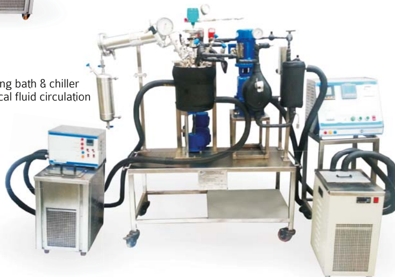
Heating cooling bath for microreactor
